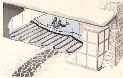
Pipes in concrete slab provide a warm floor which radiates heat to ceiling, walls, objects, people. Pipes could be in walls or ceiling.
