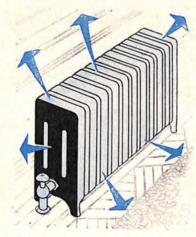
A radiator provides the greatest portion of its heat by radiant rays
