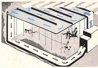
Air ducts create warm ceiling or floor panel that radiates heat to all parts of room. System can be split to provide some warm air heat
